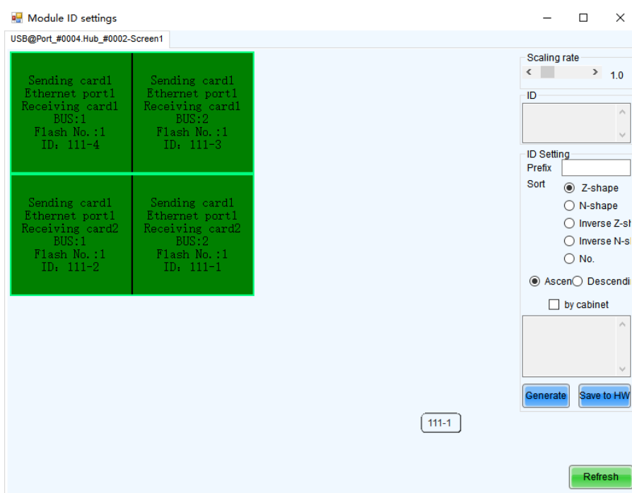
Figure 8-21 Setting module ID (regular screen)
