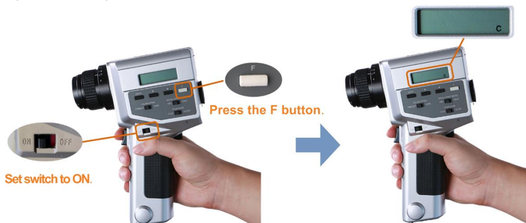
Figure 12-10 Setting CS-100A colorimeter
